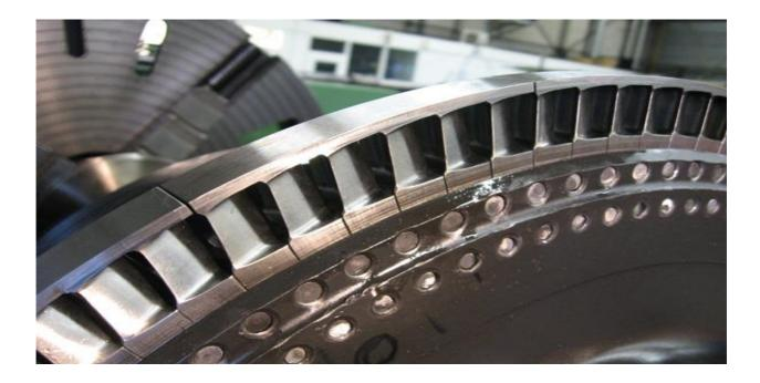
of the rotor, loss of all disc fingers over a limited circumference of the rotor and combinations of lost and intact ligaments between fingers.
