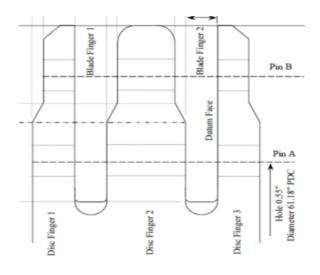
To determine the consequences of cracking of the rotor a series of scenarios were proposed. These included loss of a disc finger around the whole circumference
