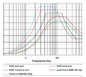
Figure 1 EUR DBEs at 0.25g and post-Fukushima SME at 0.4g (@40Hz) with 84% confidence
