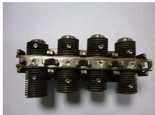
Figure 1 – Example photographs of boiler tubes Constrained within a strap arrangement.
