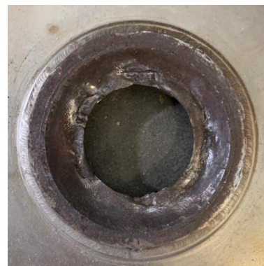
Figure 2 Failure surface of the shaft
