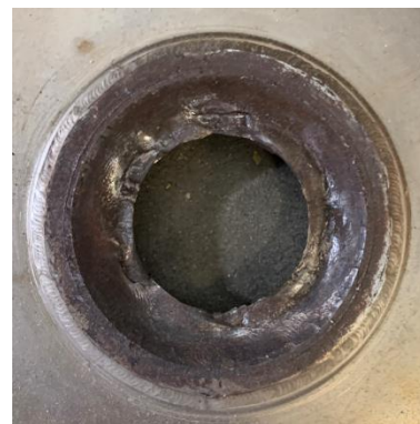
Figure 2 Failure surface of the shaft
